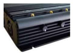
Locate the adjustable switch on the system to fine-tune the RF power output level for each band or to turn off specific bands without affecting the operation of others.
