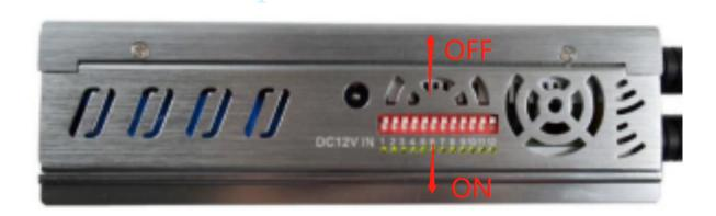
Once you've activated the Power Switch, make sure to also enable the DIP switch. The DIP switch is responsible for managing each individual antenna. Each number indicator corresponds to a specific antenna, and when the LED associated with an antenna is illuminated, it indicates that the antenna is operational.
